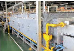
Brazing furnace with thermal insulation jacket
